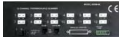
Back view; accepts any type J or K thermocouple probe with ANSI miniconnectors
